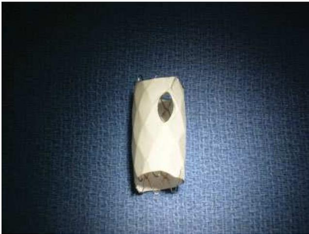
**Fig. 4.** Test perforation of e-PTFE covered stent. [Color figure can be viewed in the online issue, which is available at [www.interscience.wiley.com](http://www.interscience.wiley.com).]
